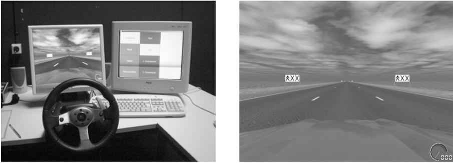
**Fig.1. Experimental setup on the left, the drivers view on an indicated lane change on the right**
