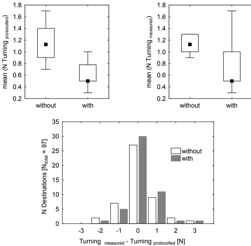
**Fig.2. Influence of navigation system on measured (upper left) and protocolled (upper right) turning manoeuvres. The lower graph shows the absolute difference between measured and protocolled turning manoeuvres per destination reached.**
