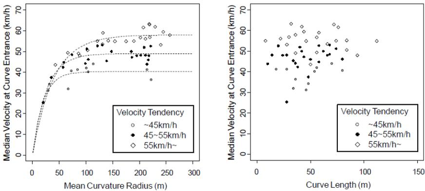
**Fig. 4. Entrance Velocity and Velocity Tendency at Curves**
