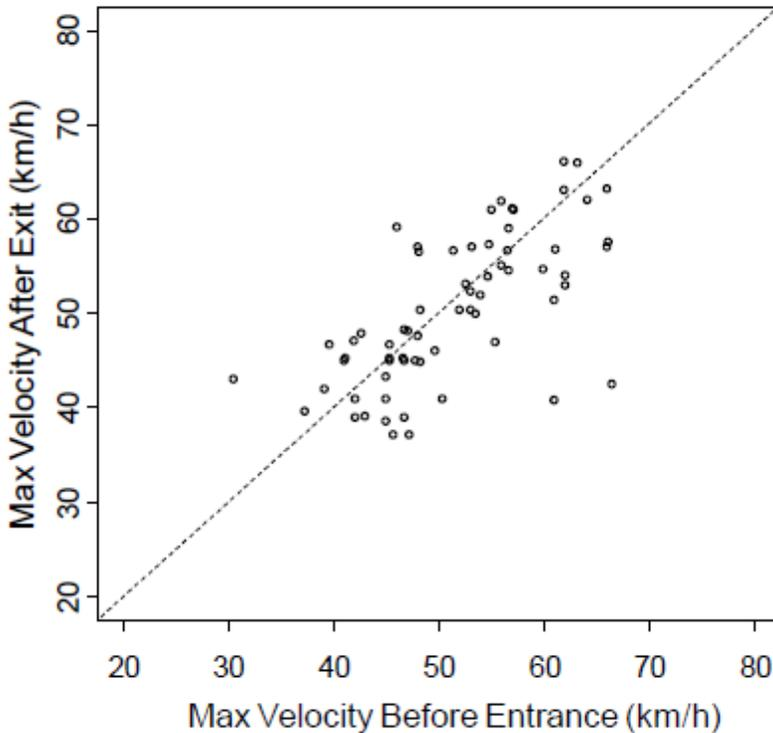
**Fig. 6. Peak Velocities Before and After a Curve**
