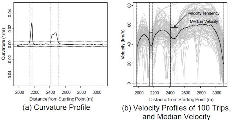
**Fig. 1. Curvature and Vehicle Velocity on a Road Segment with Two Curves**
