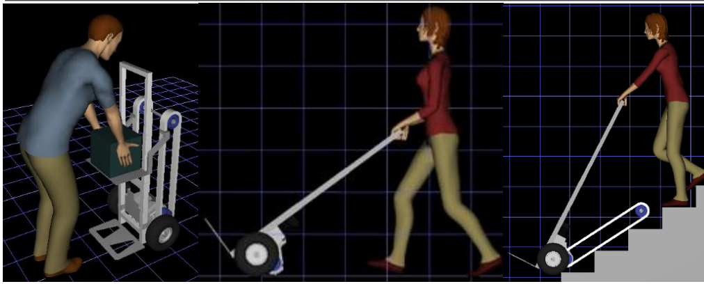
Figure 1 Simulation of the three main functions: actuated moving tray for loading- unloading, traction wheels for uphill and downhill transportation, stair climbing
