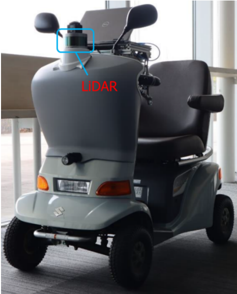
Figure 1 – Automated driving mobility scooter
