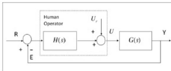
**Fig.2. Control theoretic model of human operator from [10]: R=Reference input, E=Error, Y=Output variable, U=Control variable, Ur=remnant**
