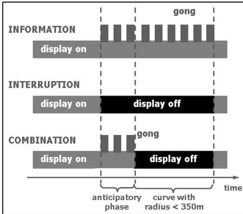
**Fig. 2: Schematic description of the functionality of the conditions "information" (top), "interruption" (middle) and "combination" (bottom) during the anticipatory phase and the curve. The gongs are displayed as vertical bars, the activation of the system is labelled as colour (grey: display turned on; black: display turned off).**
