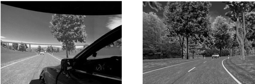
**Fig. 1: High-fidelity driving simulator of the Wuerzburg Institute for Traffic Sciences**
