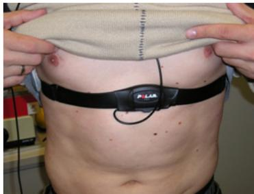
**Figure 2: Heart rate measurement device for use while riding a motorcycle**
