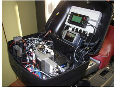
**Figure 1: Measurement equipment in the topcase of the motorcycle (from Haumann et al., 2006)**
