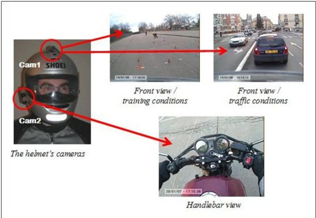
**Figure 3: Cameras mounted on the rider's helmet (Aupetit, S., Riff, J., Buttelli, O, & Espié, S. (2008)**
