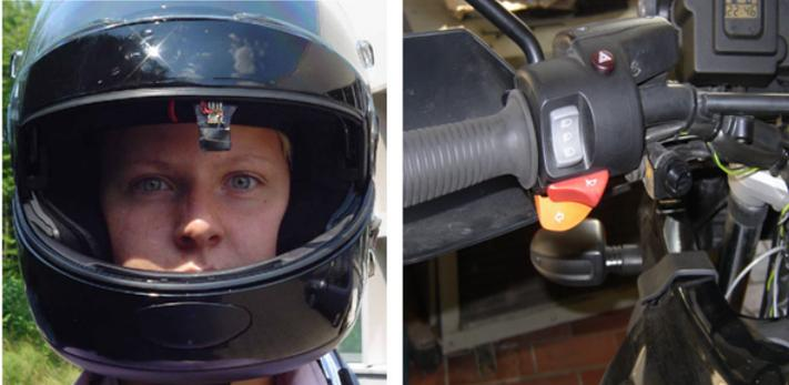
**Figure 4: Apparatus of the PDT modified for the measurement of rider workload (from [3])**
