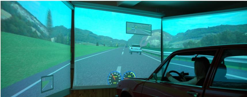
**Fig.2. CRISS Driving Simulator: phase of the experiment**
