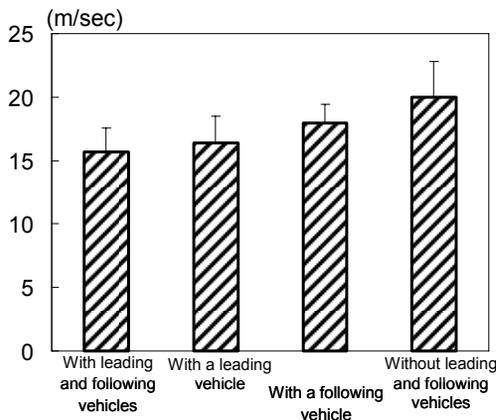
Fig.4. Average driving speed when covering the brake pedal in the four traffic conditions
