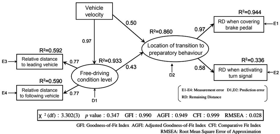
Fig.5. Path diagram of the constructed structural equation model
