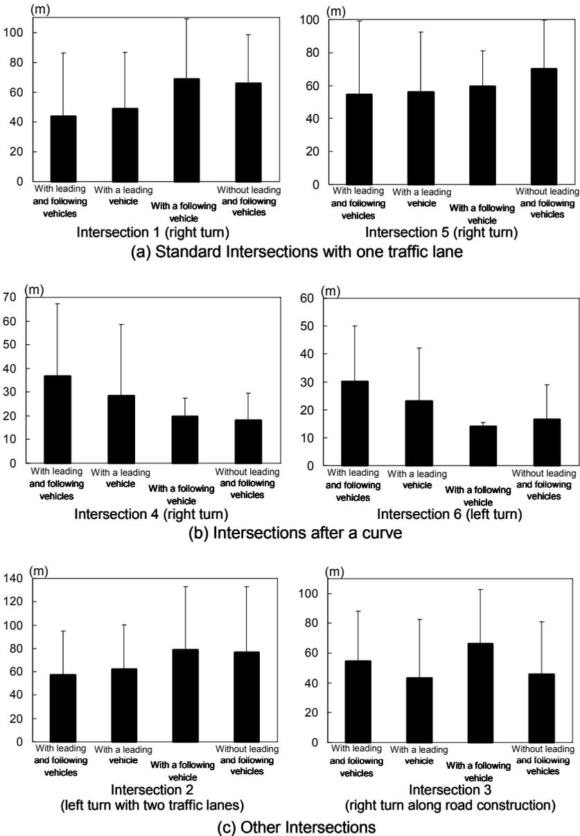
Fig.7. Average onset locations of covering the brake pedal on the analyzed intersections
