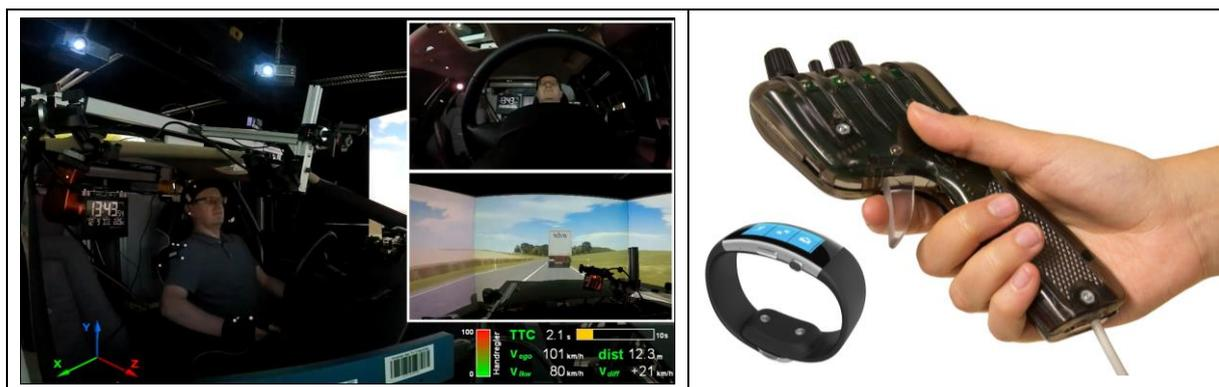
**Figure 1 – Driving simulator study setup in the truck approach situation (left), smartband Microsoft Band 2 and handset control for continuous discomfort assessment during automated driving (right)**
