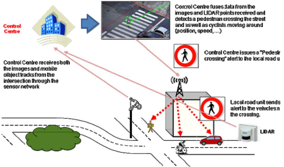
Fig. 2 Automatic detection of pedestrians and other VRUs on the road
