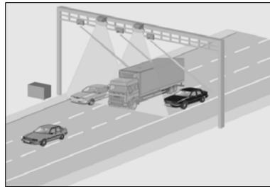
**Fig.2. Laser sensor**
