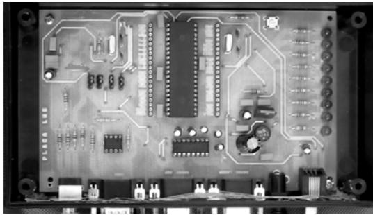
**Fig.3. Control and communications card**
