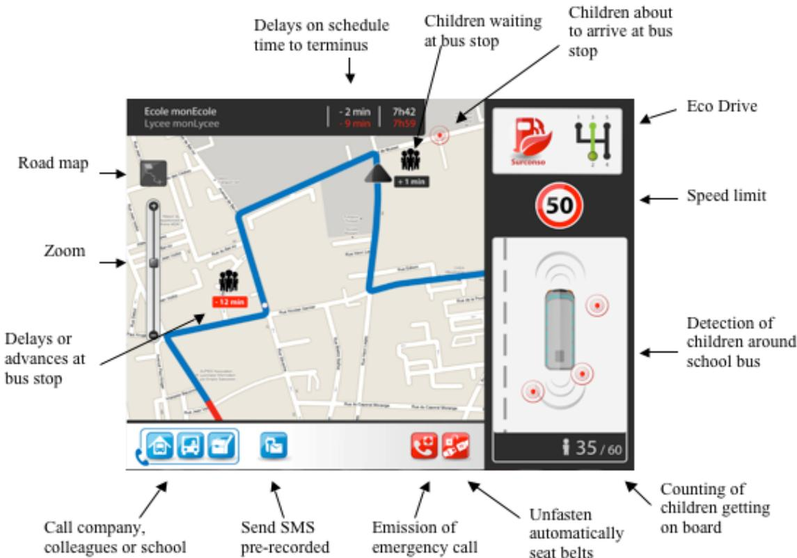
**Figure 2: Functionalities implemented in the DSS ergonomic mock-up developed in the framework of Safeway2School project**
