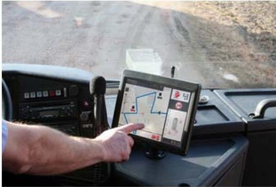
**Figure 3: Test of ergonomic mock-up usability and acceptability by school bus drivers**
